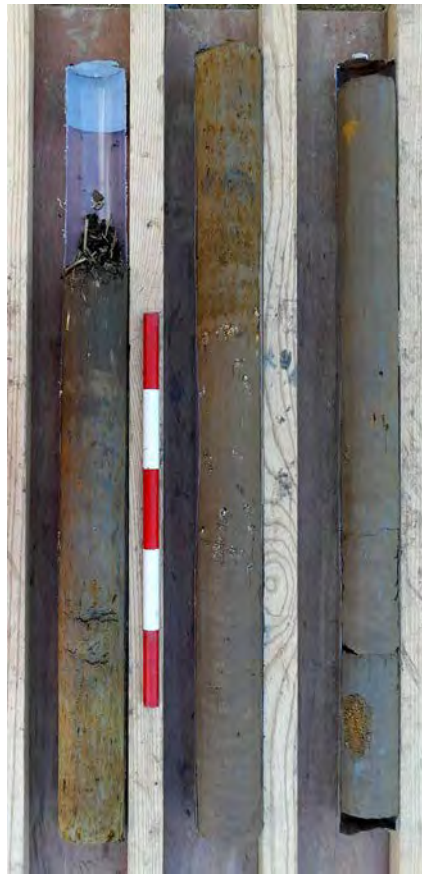
Plate 11: Weathered bedrock overlain by brickearth and a thin alluvium, Borehole OCA-WS201A, 0-3m, Transect 2 (ground surface, top left)
