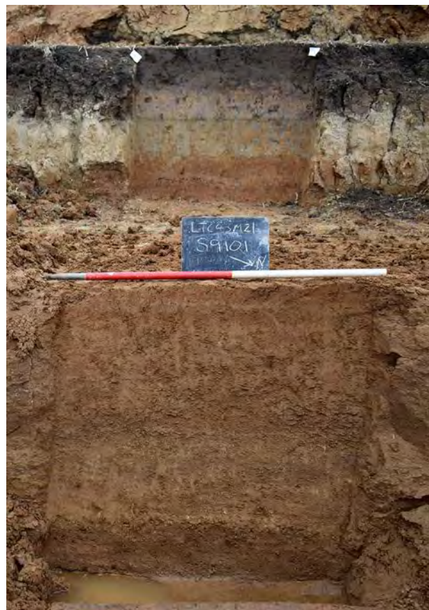
Plate 26: Basal sand and gravel overlain by brickearth and capped by alluvium, Section 9100, Trench 91, Transect 14. Note the leached horizon at the top of the brickearth
